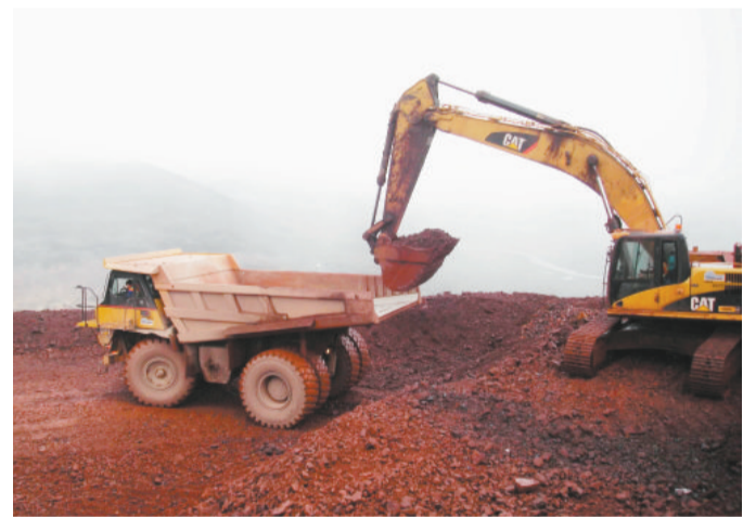
A backhoe loads ore during bulk sampling at the Baffinland Iron Mines Corp Mary River project last month.
